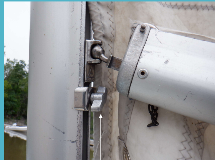
Butterfly nut: Adjust height of the boom
