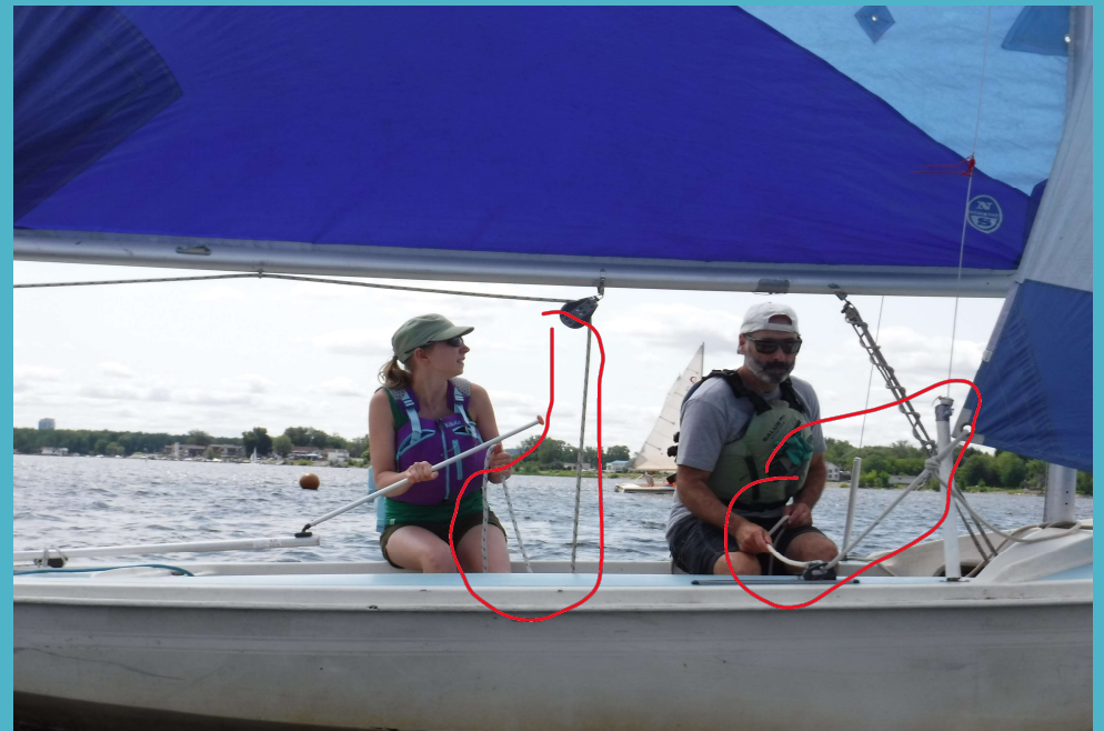
Control/trim the jib and main: jib sheets (x2) and mainsheet (x1)
